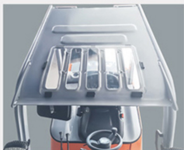
一体冲压成型顶架，透明PVC顶棚，防落物，防雨淋，视野清晰，安全可靠 One stamping molding protection frame, transparent PVC ceiling, anti-fall, anti-rain, clear vision, safe and reliable.
